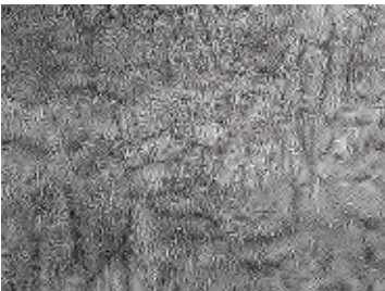
Figure 1: Acceptable microstructure of castings (100X) (1)
