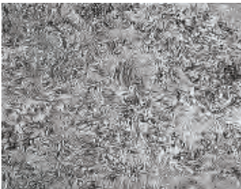
Figure 1: Acceptable microstructure after welding (100X) (1)
